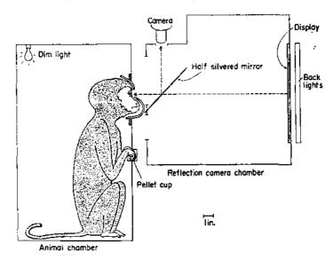
FIG. 3. Diagram of the recording apparatus and animal chamber.
