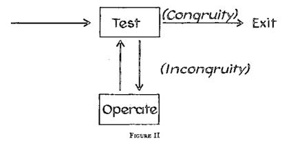
The TOTE (Test-Operate-Test-Exit) unit, a feedback alternative to the reflex arc. Note that exit occurs when matching or congruity is achieved in the test phase, and not as a consequence of the operation or action per se.
