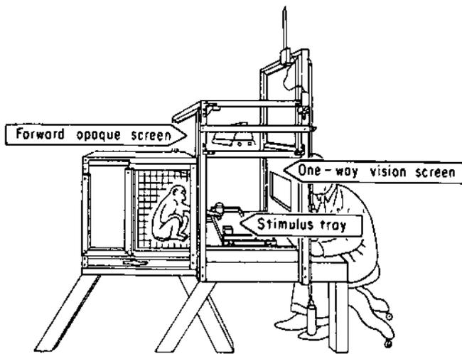
FIGURE 6 Wisconsin General Testing Apparatus (WGTA). Used to test monkeys in a variety of discrimination and learning problems.
